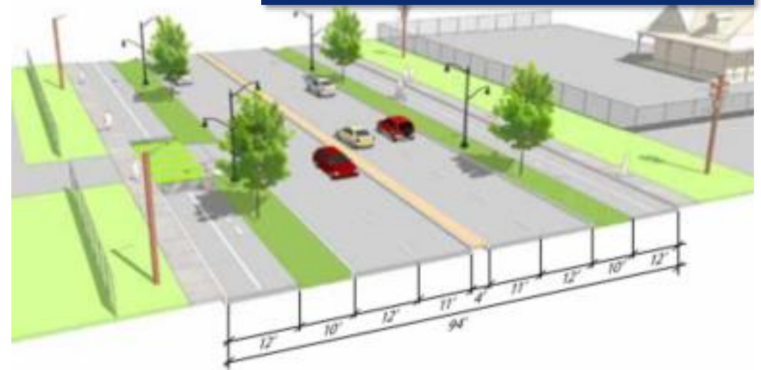
Example Cross Section from Route 9 Master Plan
